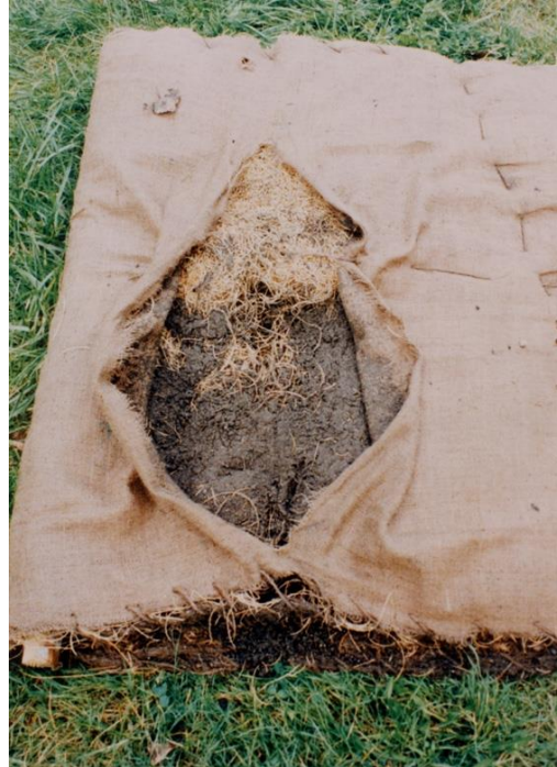
Plate 6 "Full" Sedimat after having been removed from stream bed
