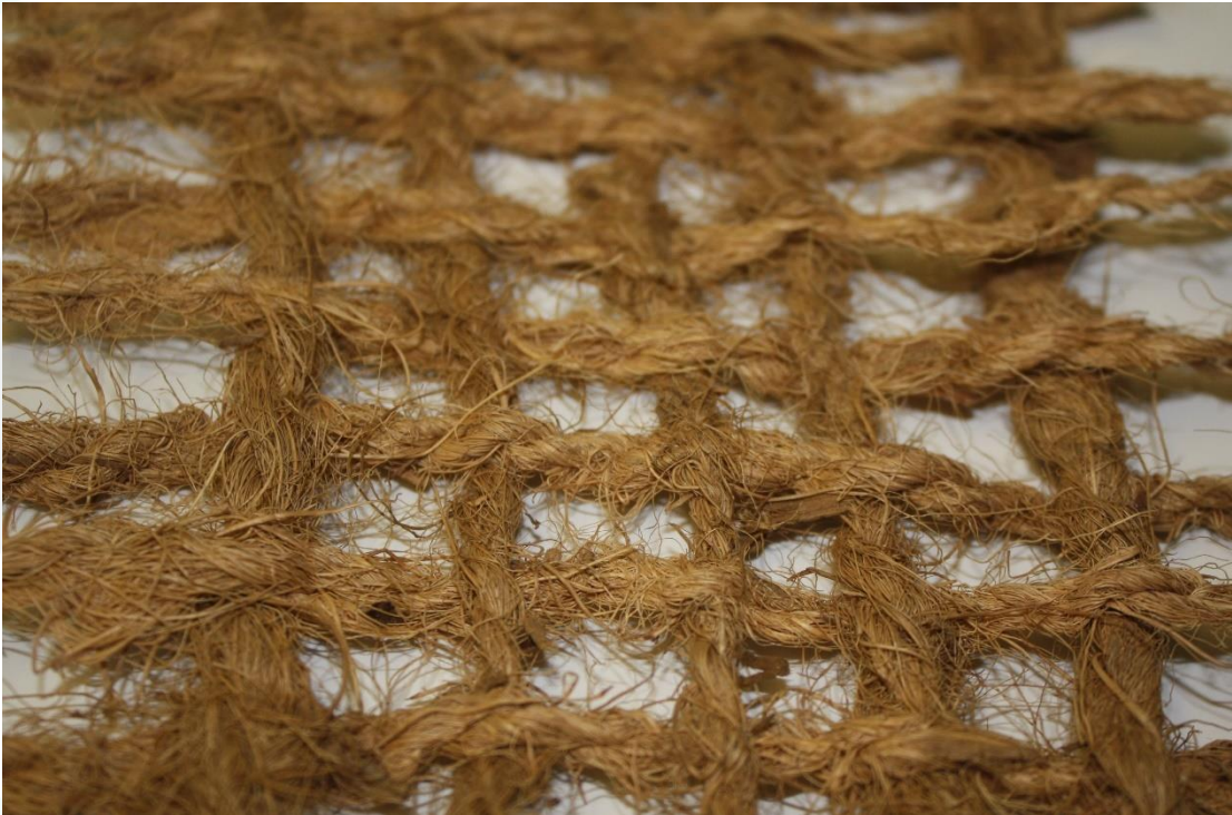
Plate 2 CoriMesh biodegradable woven coconut fibre used on bare surfaces to prevent erosion and promote revegetation
